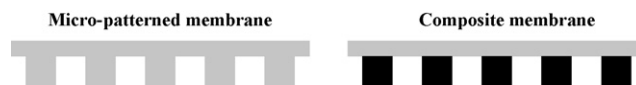
Fig. 6. Schematic representation of the cross-section of a micro-patterned membrane (left) and a composite membrane (right) with the same dimensions.
