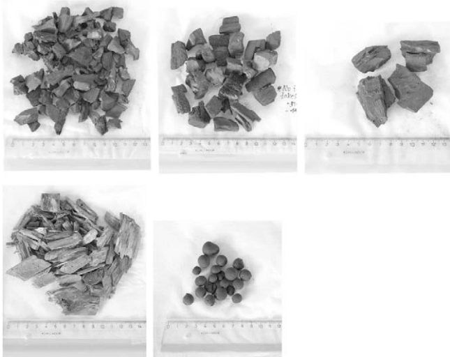
Fig. 3. Some of the used fuels. Upper left to right: small char (10–15 mm), medium char (15–30 mm), large char (30–40 mm). Lower left to right: wood chips (10–40 mm), stones (10 mm).
