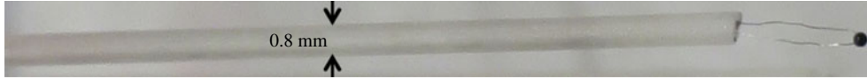
FIGURE 2. Photograph of a Honeywell 111-104HAK-H01 thermistor assembled with its 0.8 mm diameter ceramic rod, ready for insertion into the interior of the cell.
