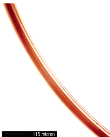
Figure 1. Flexible fiber drawn from melt polymer 13 .
