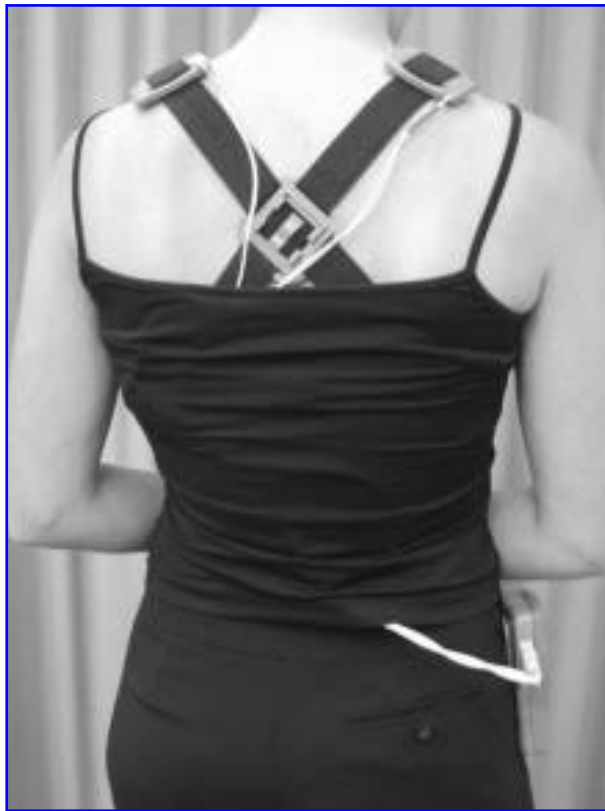
FIG. 1. The myofeedback harness with dry sEMG electrodes.
