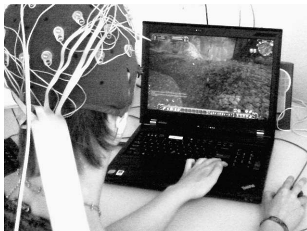
Fig. 6. A user playing World of Warcraft using both conventional controls and brain activity to control her character in the game.
