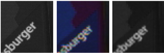
Fig. 3. Comparison of the AVT Stingray F-046B monochrome camera with shutter 1/60s (left) to the AVT Stingray F-046C Bayer colour camera with shutter 1/20s (middle). The right image is obtained by converting the colour image to a grey image.
