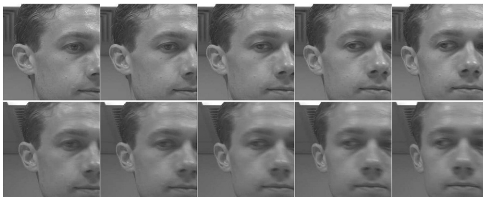
Fig. 4. Example of two trade-offs between shutter time and aperture. The recorded action is a quick head turn as the result of a sudden change of attention. The images are cropped at 300 \times 300 pixels from a full resolution of 780 \times 580 pixels. The top row shows 5 subsequent images taken at 60 fps, with a shutter time of 5 ms. The bottom row shows images taken at the same moments, from a synchronised camera, with a shutter time of 15 ms and a smaller aperture, to obtain the same image brightness. The result of the longer shutter time is an increased motion blur, while the smaller aperture results in a sharper background due to the increased DoF.
