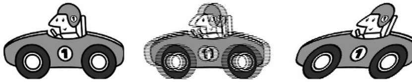
Fig. 2. Example of how an image of a horizontal moving object looks like, when captured with a camera with (1) progressive scan with global shutter (left), (2) interlaced scan (middle) and (3) progressive scan with rolling shutter (right).
