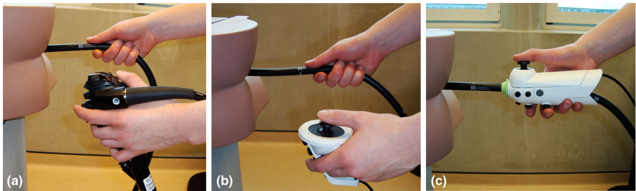
Fig. 3 Test configurations. Each group of participants used either the conventional (a), bimanual joystick (b) or single-handed joystick (c)
