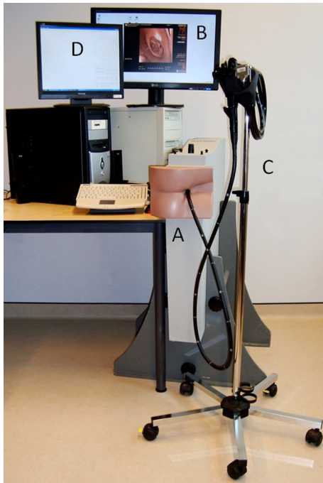
Fig. 4 Experiment setup, with A the virtual endoscopic computer simulator, B endoscopic image, C holding standard (when using bimanual and single-handed joystick interfaces) and D a screen with feedback diagram
