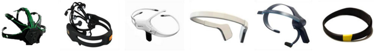
Figure 1. Current wearable BCI devices (from left to right): OpenBCI 3D printed EEG headset, Emotiv EPOC, Emotiv Insight, Interaxon Muse, Neurosky Mindwave, Melon.
