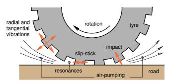
Figure 2: Mechanisms of tyre/road noise generation.
