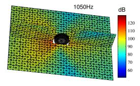
Figure 3: Sound pressure level at 1050 Hz of a slick tyre on a flat, acoustic hard road (the tyre rolls to the right) [2].
