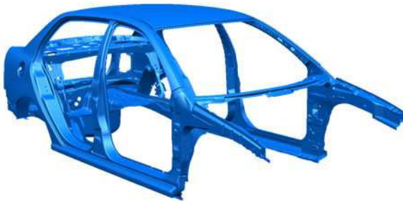
Figure 1 : Car body inner and outer panels.
