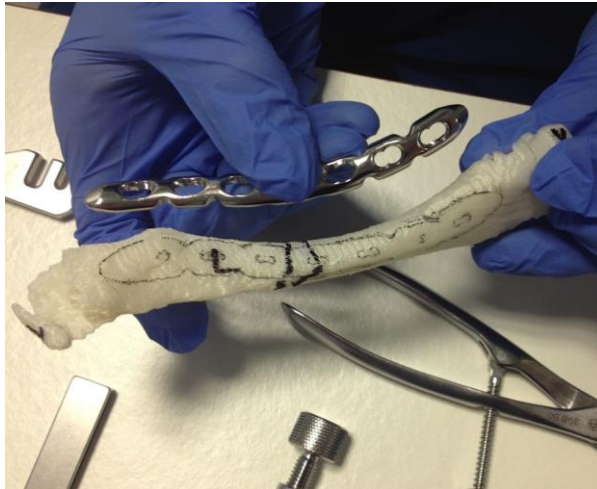
Figure 3. The mirrored contralateral model of the pilot case and the resulting fixation plate after bending.
