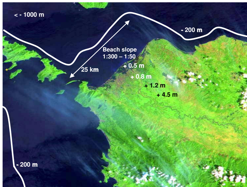
Figure 3. Summary of findings on coastline, bathymetry and topography of Banda Aceh beach before the tsunami, overlaid on a satellite image of the area.
