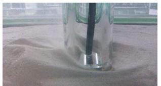
Figure 1. Initiation of scour hole formation during experiment
