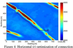
figure 4: Horizontal (r) optimization of connection between two wind turbines
