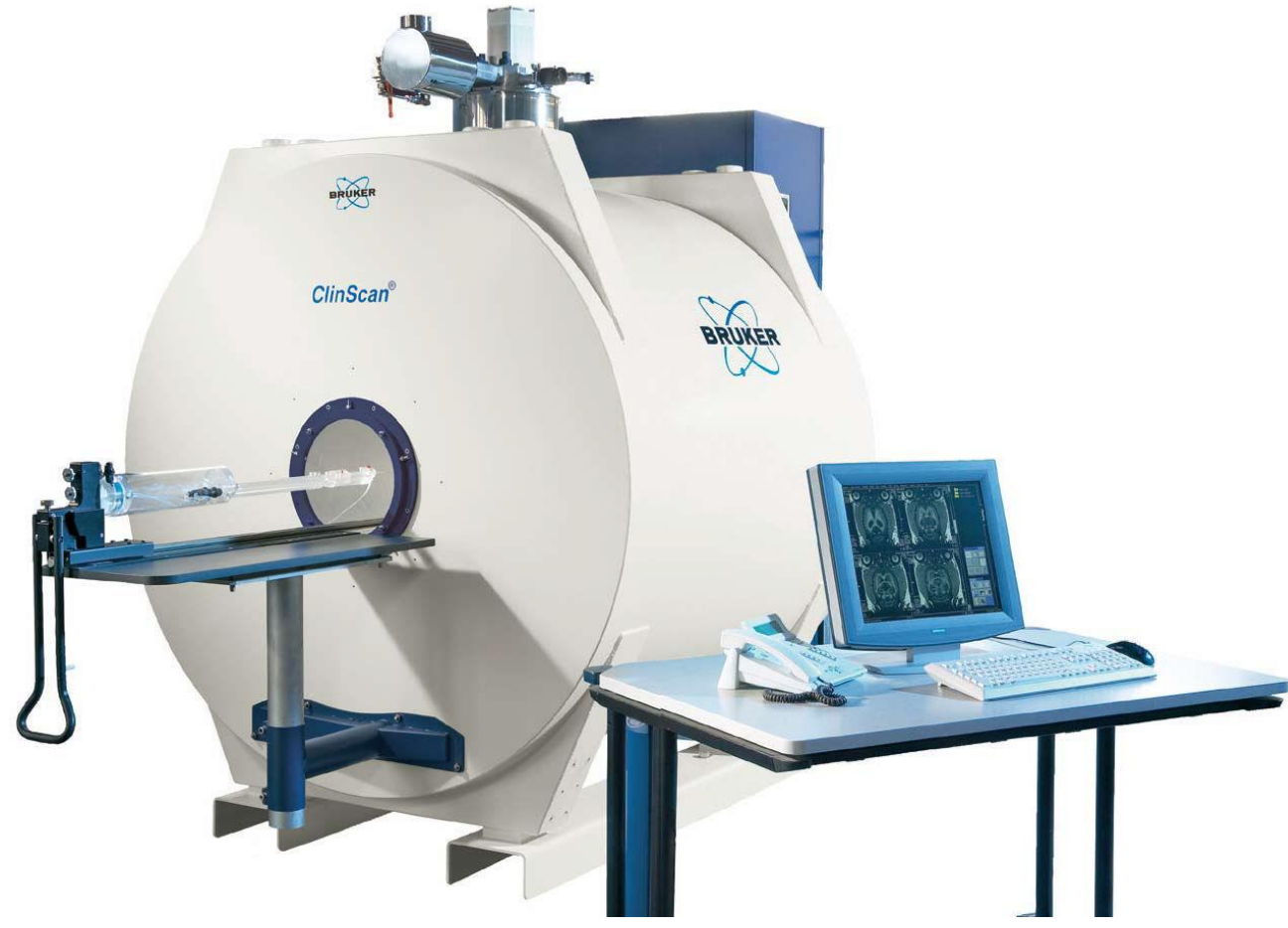
Figure 1. Image of Bruker's 7T small animal MRI scanner [5].
