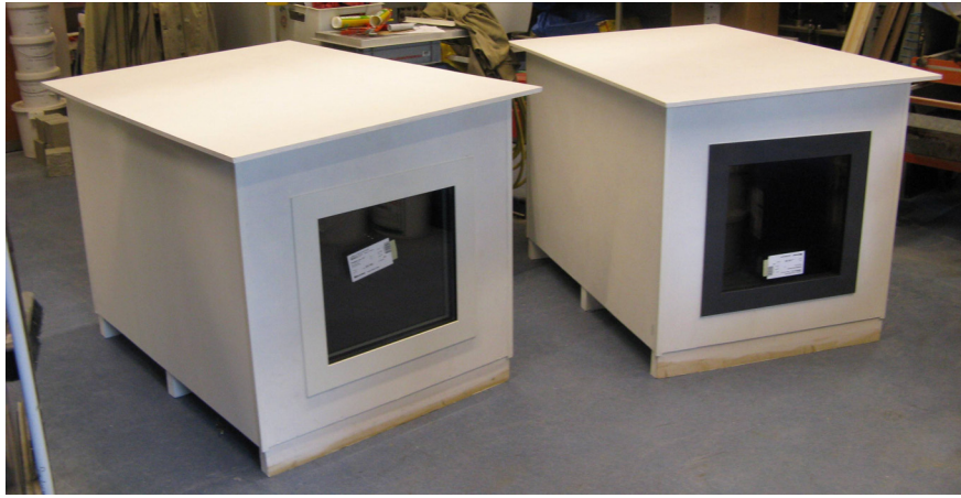
Figure 1 Two boxes for the experiment, one with PCM and one without PCM in the concrete floor
