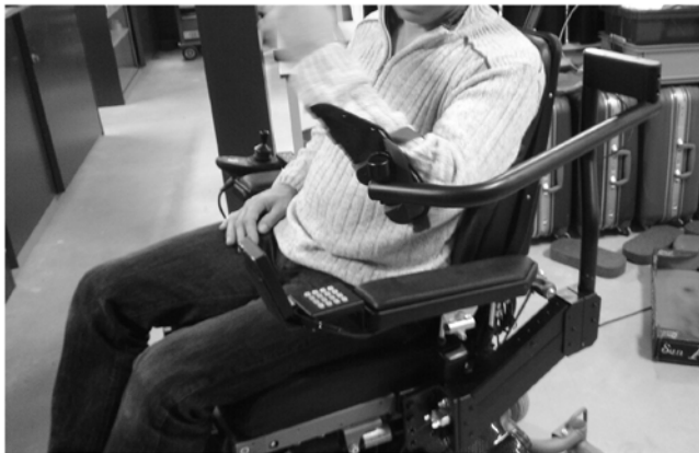
Fig. 4. DAS prototype with arm cup including straps on a wheelchair
