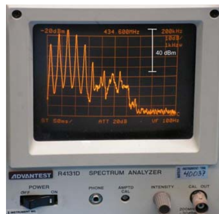
Figure 32. TM transmitter interference test result
