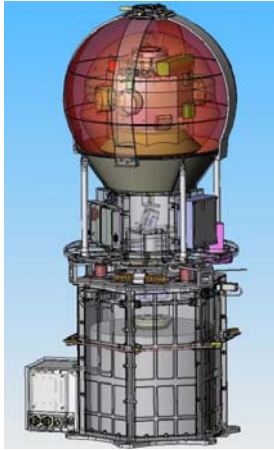
Figure 1. YES2, from top to bottom: Fotino re-entry capsule, tethered MASS sub satellite, FLOYD tether deployed.
