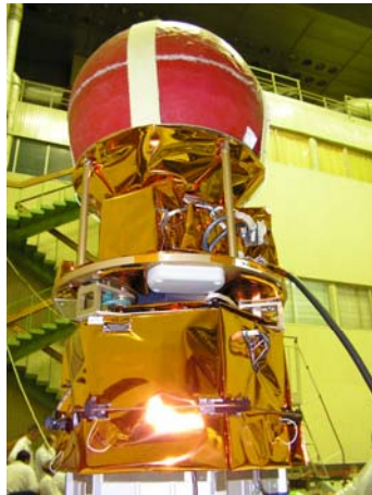
Figure 26. Bottom view of YES2, MASS GPS/GLONASS antenna (large white, middle) and MASS UHF TX antenna (yellow, mid-left) are visible.
