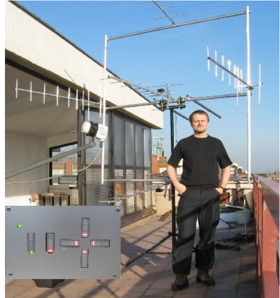
Figure 27. Portable ground station for Fotino telemetry reception and tracking (4 tracking yagi's and a central main receiving yagi).
