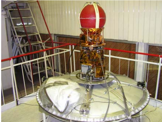
Figure 25. The diametrically placed GPS/GLONASS antenna's and combiner of the YES2 SSAU experiment are visible on the Foton plate at the bottom of YES2. Also visible is the late addition of MLI for extra thermal insulation that blocks the FLOYD receiving hexagonal antenna and heavily reduces its performance.
