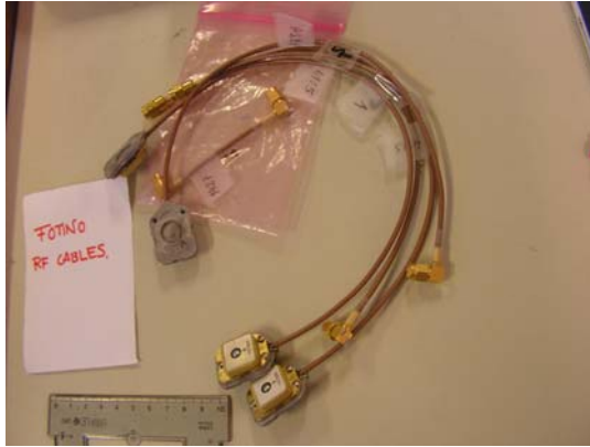
Figure 17. GPS antenna's prepared for installation on Fotino
