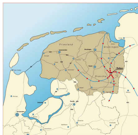
Figure 1. Geometrical overview of LOFAR. All the red dots are stations.
