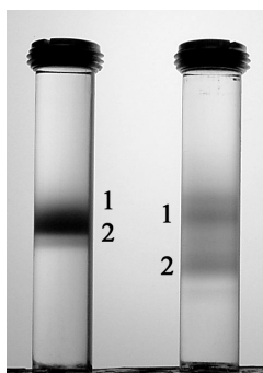
Fig. 2.7. Solubilization of LH2-only membranes with DDM with subsequent fractionation by ultracentrifugation on sucrose density gradients. On the left: membranes solubilized with 0.005% DDM, on the right: membranes solubilized with 0.01% DDM [Image courtesy of John Olsen, University of Sheffield].
