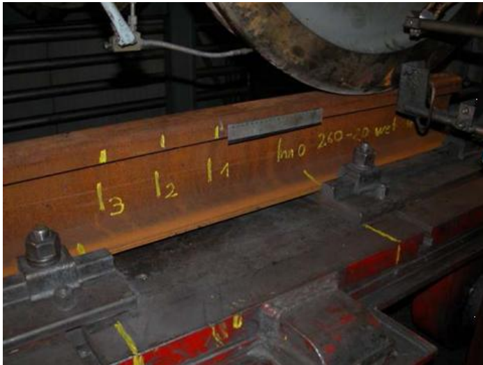
(b) The rail and wheel test rig.
