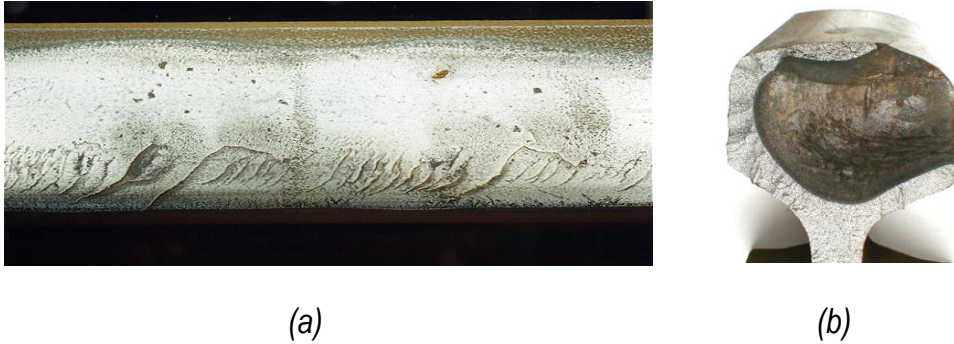
Figure 1.1 Severe Head Checks (a) and cross section of a severe single Head Check (b).
