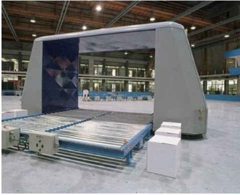
Figure 3.4. One of the prototype vehicles while docking: the Lödige vehicle (Rijsenbrij et al., 2000)
