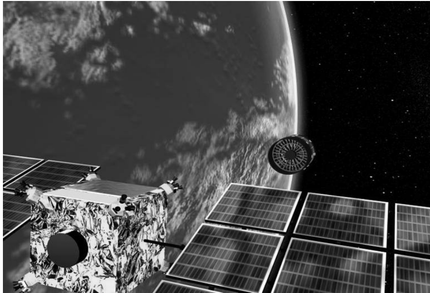
Figure 1.2: Artists impression of the XEUS spacecrafts in their final configuration with the mirror and detector spacecraft separated by 50 m.
