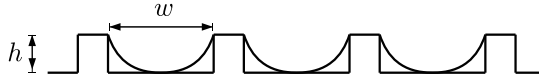
Figure 2.7: Touchdown scenario. The liquid-gas interfaces are assumed to collapse when they touch the floor of the texture.
