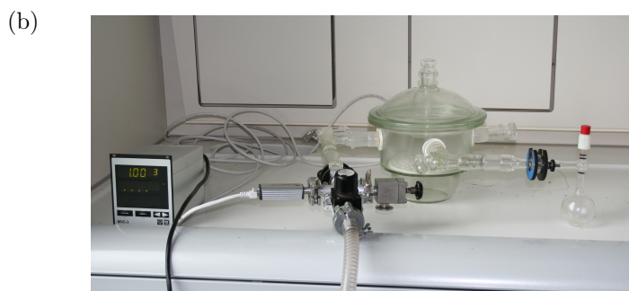
Figure C.1: Schematic (a) and photograph (b) of the setup for controlled vapor deposition of an alkylsilane.
