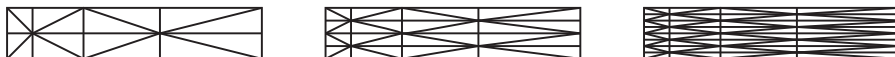
Figure 7.4: The used different mesh densities: coarse (left), intermediate (middle) and fine (right). The sample models 2 mm length and 10 mm width, with the free edge on the left.
