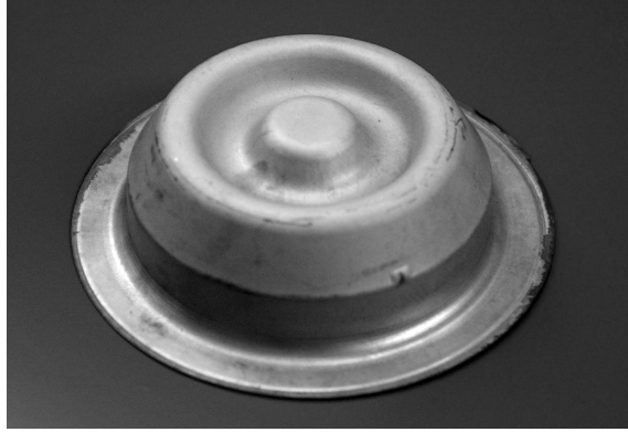
Figure 3.20: Photo of a formed sheet as a result of the die bulge experiments.
