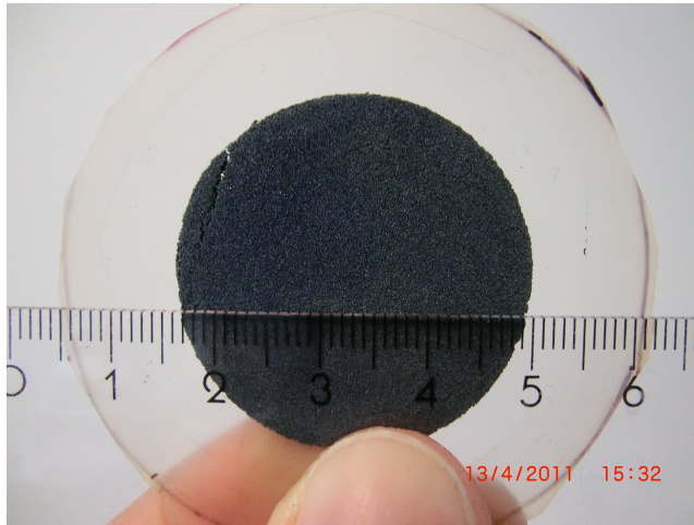
Figure 3.4 MEA for the charging procedure of the Modular Vanadium/Air-RFB, a Nafion-117 membrane hotpressed under a pressure of 2.34\text{kN/cm}^2 for 15 minutes to a porous sintered titanium (thickness= 1mm; \text{Ø} = 33 mm; porosity= 45%) electrode coated with Pt/Ir (70/30 wt%).
