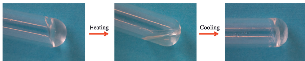
Figure 4. Vial tilting of 1800-HPEI-8.2-(PLLA-mPEG) 2 copolymer (27.5 wt %, PBS pH7.4). Upon heating a gel-sol transition takes place at 68 °C and upon cooling a sol-gel transition takes place at 64 °C.
