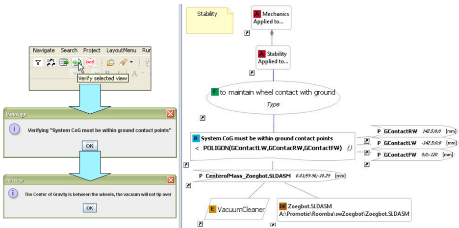
Figure F.9: Verification: Knowledge bases can be developed to perform specific verification tasks. In this case, the user is informed of the system is still mechanically stable.
