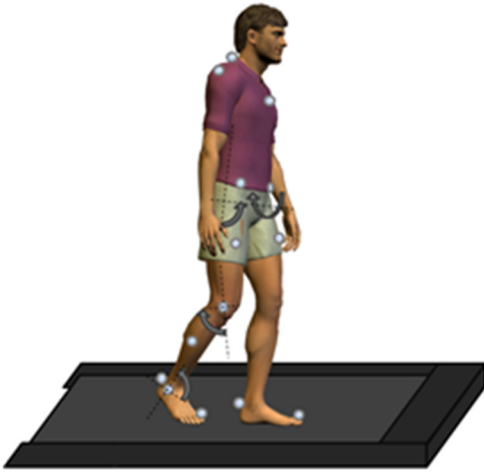
Figure 1: Marker placement. To track the motion of the subject, twenty one passive reflective markers (gray circles) were attached to bony landmarks and segments on the legs and trunk. Joint angles are defined according to the classical method used in clinical examination, where (dorsi-) flexion and abduction are defined positive.
