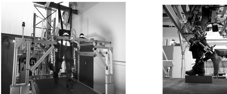
Figure 1: Left: The LOPES robotic gait trainer. It comprises a bilateral exoskeleton series elastic joints, actuated via Bowden cables and capable of applying torque perturbations to the hip and knee joint. Right: Experimental setup. During the perturbation experiments the subjects stood with the non-perturbed leg on a box such that the perturbed leg could move freely.
