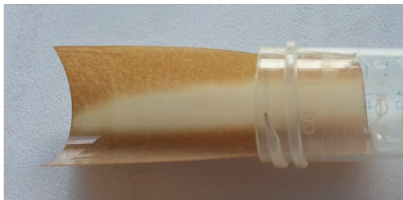
Figure A7-6. PAN supported pepsin membrane after 29 hours of contact with hemoglobin in solution at a temperature of 37 °C and pH 2 (HCl adjusted). The brown color originates from the hemoglobin digestion products that are adsorbed into the membrane layer.
