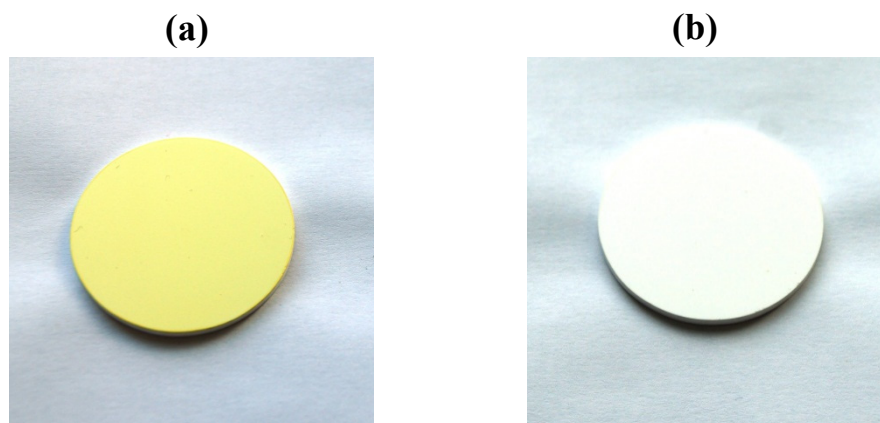
Figure 3.4 Photos of a SPEEK film \sim 800 nm with a DS of 84 % coated on a \gamma/\alpha -alumina support (a) directly after incubation at a 60 °C in a vacuum oven and (b) after few minutes in a humid atmosphere.
