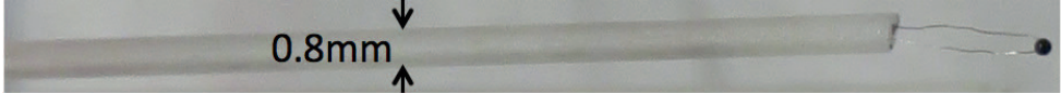
Figure 2.2: Photograph of a Honeywell 111-104HAK-H01 thermistor assembled with its 0.8 mm diameter ceramic rod, ready for insertion into the interior of the cell.
