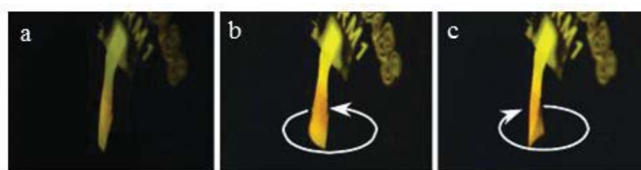
Figure 2.15 a) Strip film before light illumination. b) and c) Twisting of strip films with counter-clockwise and clockwise turn under -45^\circ and 45^\circ polarization relative to long axis of strip, respectively. Adapted with permission from [84] (Copyright 2005 Optical Society of America).
