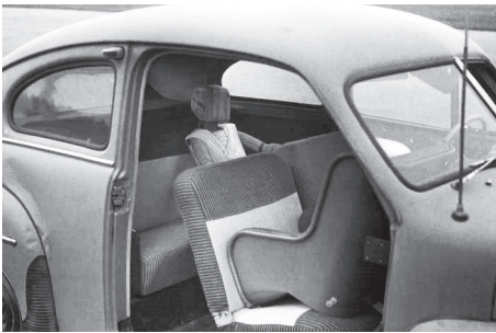
Figure 7.4. Prototype of a first rearward facing CRS tested in 1964 (Volvo, 2014).
