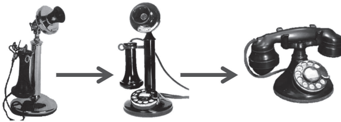
Figure 4.3. Evolution in early telephones: at system level operator networks were replaced by pulse network, the second-order subsystem rotary-dial was introduced and then the designs of second-order subsystems like dial and handset were further integrated.
