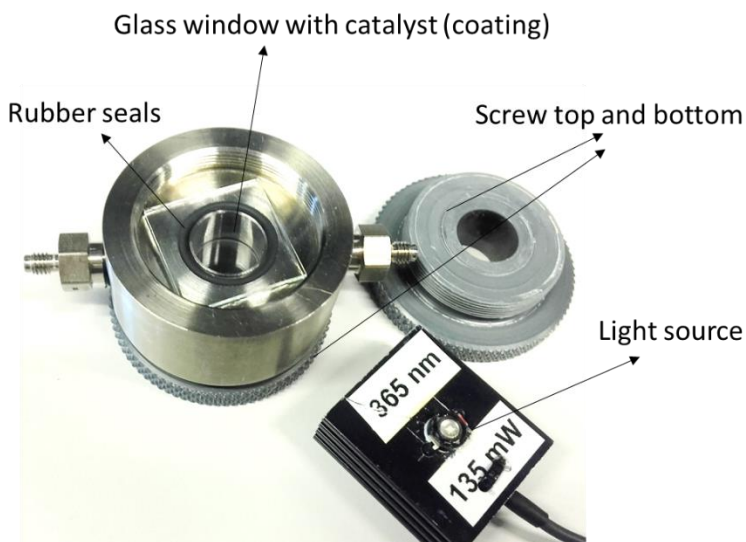
Figure 3: Image of the top illuminated batch reactor used.
