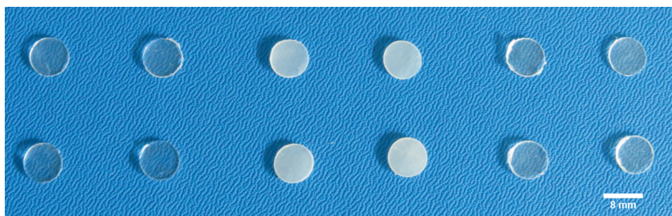
Figure 6.5: \varnothing 8 mm PTMC discs (left 4), PTMC discs with GEN-SULPH (middle 4) and PTMC discs with GEN-AOT (right 4) prepared by compression molding.
