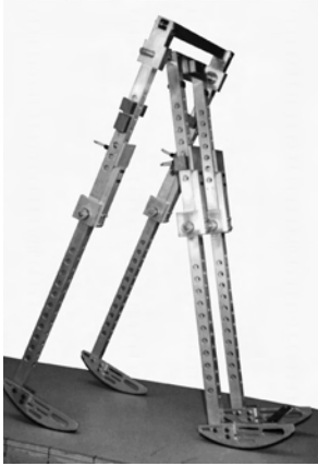
(a) Close copy of McGeer's passive dynamic walker, by Garcia et al. (1998).
