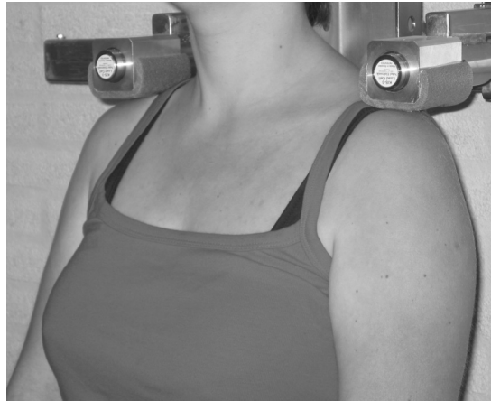
Figure 5.2 Measurement set-up with the two force transducers located slightly above the acromion at both sides. Force and EMG (not visible) were measured simultaneously from the trapezius muscle. Force feedback was provided on a laptop in front of the subject.
