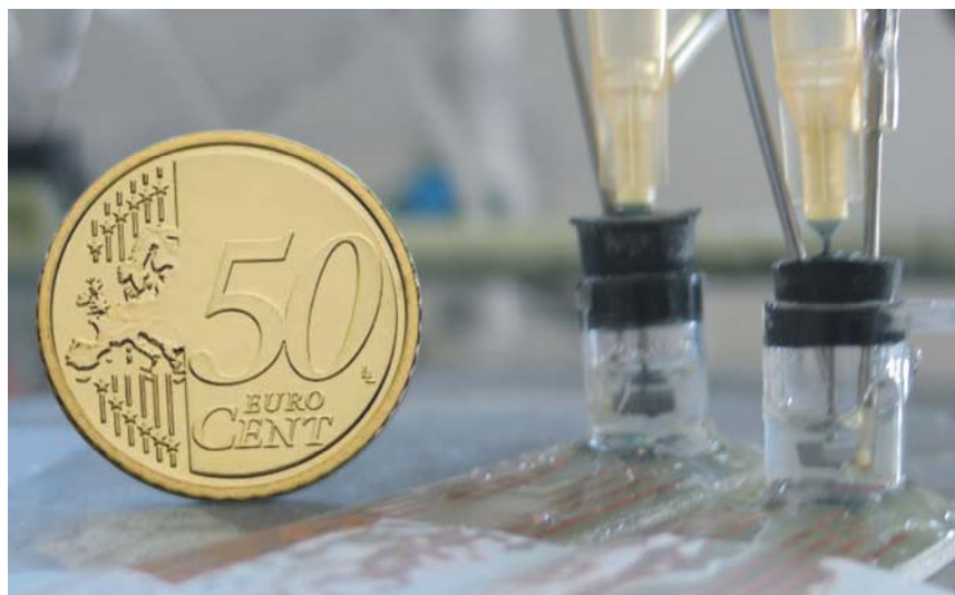
Figure 6-3: closeup picture of two micro bioreactors, the coin on the left has a diameter of 25 mm
