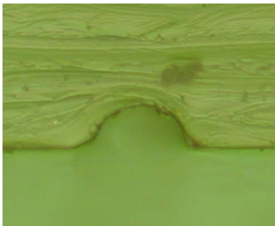
Figure 7-4: Cross section of PDMS microchannel
