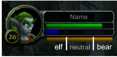
FIGURE 9: Orange feedback bar with thresholds. The user has to go below 0.3 to change to elf, and above 0.7 to change to bear. In between no action is performed.
