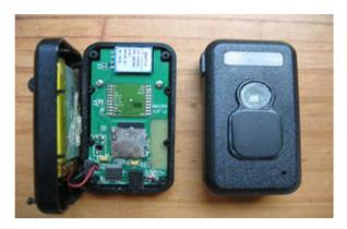
Figure 1-1 The custom designed wireless sensor node used to collect PS dataset
