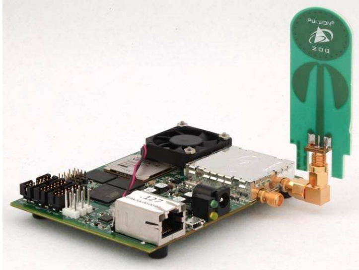
Figure 2.6: Time Domain Broadspec UWB antenna attached to a P400 RCM ranging and communication module.
