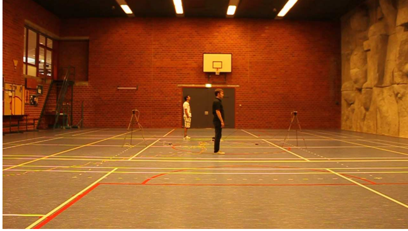
Figure 5.3: UWB setup for multiple people detection and localization measurements.
