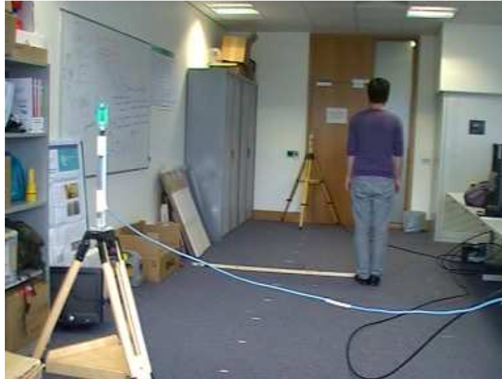
Figure 2.8: An example measurement scenario during the laboratory measurements: the subject is positioned on the fourth vertical (T4) and ninth horizontal position (H9) in a perpendicular orientation, with an antenna separation of 7 m.
