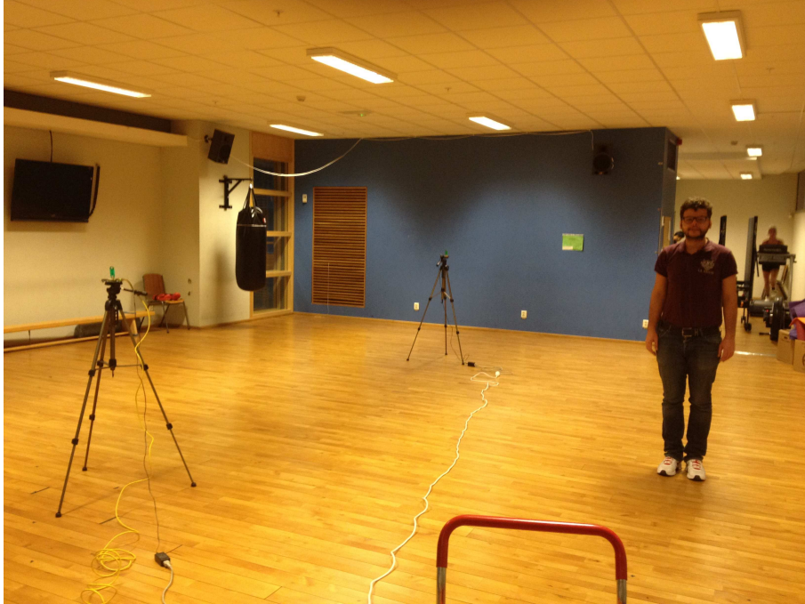
Figure 3.11: UWB setup for device-free detection and ranging measurements. The person is standing at H1 (see Fig. 3.10) with a perpendicular body orientation.
