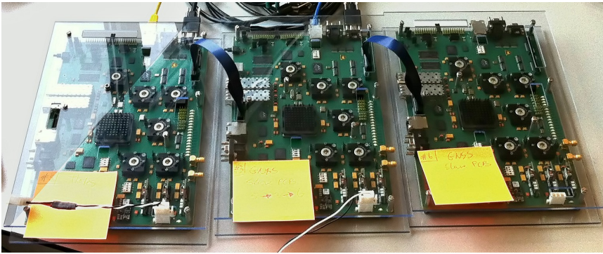
Figure 4.13: A GSP instance composed of three boards totaling 146 cores.
