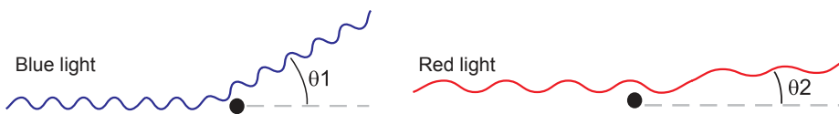
Figure 2.9 Rayleigh scattering is caused by particles smaller than the wavelengths of light and is greater for small wavelengths.
