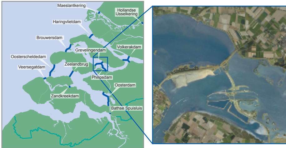
Figure 12.7 Dutch Delta Works to protect the heavily industrialized and densely populated western part of the Netherlands. Blue bars in the left-hand image are barrier constructions, such as the Philipsdam shown in detail on the right. Source: left [27], right [40].
