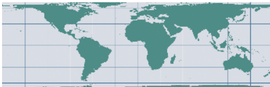
Figure 3.20 The cylindrical equal-area projection, i.e. a cylindrical map projection with equal-area properties. Distortions of shapes are significant towards the poles.
