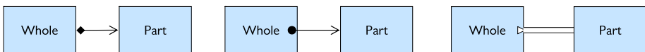
Fig. 12. “Piercing” elements (middle) conveys the concept of being “part of” in a more perceptually direct way than the existing convention (left) and makes such relationships more discriminable from other types of relationships. A “dovetail joint” (right) provides another possible option.
