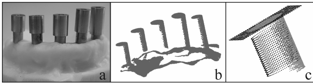
Figure 3: Measurement of position of implants: (a) registration elements mounted upon implant replicas of work model, (b) point cloud of scanned elements, (c) fit of top plane and cylinder surface on identified points of a registration element.
